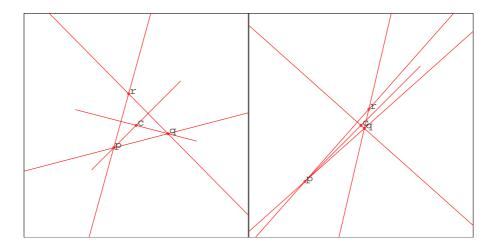
Figure 3: 2D system of 4 points and 5 lines with 10 point-line incidences, 4 angle parameter  $\operatorname{angle}(qp,cp)$ ,  $\operatorname{angle}(cp,rp)$ ,  $\operatorname{angle}(rq,cq)$ ,  $\operatorname{angle}(cq,pq)$  and 1 distance parameter d(r,c). Symmetric solution (left) and random, typical witness solution (right).
