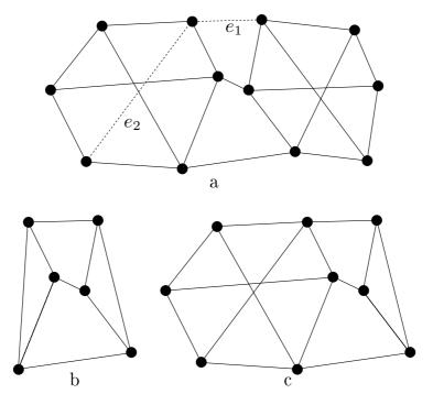
Figure 8: 2D systems where edges represent point-point distances; a: 3-connected constraint graph made of two  $K_{3,3}$  graphs connected with 3 constraints; b and c: graphs obtained by replacing MRSs identified by algorithm 3 by their boundary with respectively edges  $e_1$  and  $e_2$  removed.
