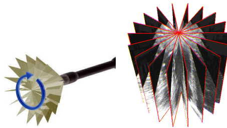
Figure 5: A rotative ultrasound probe and the resulting cylindrical geometry image. This image was acquired at the CHU Brabois by Dr Lethor for the Échocard3D project.
