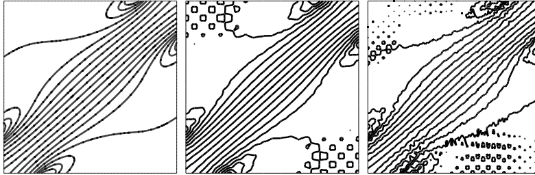
Figure 7: Stream lines: fine regular mesh (left), regular 20 \times 20 grid (middle), irregular grid (right)
