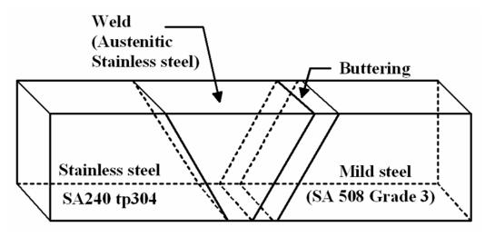
Fig.2 Description of the Dissimilar Metal Weld
