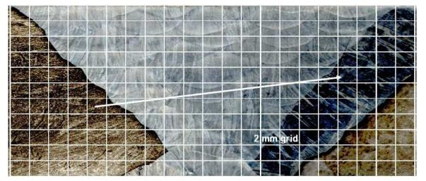
Figure 1: Macrograph of a real specimen, with buttering
