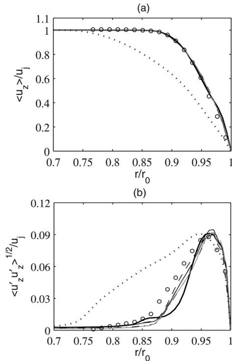
FIG. 5. Profiles at  $z=0$  (a) of mean axial velocity  $\langle u_z \rangle$  and (b) of the rms values of fluctuating axial velocity  $u'_z$  for — (thick line) Jetnoise256, — Jetring256, - - - Jetring256drdz, - · - · - Jetring512, gray solid line: Jetring1024dz, gray dashed line: Jetring1024drdz, and ····· Jetring1024drdz $2\delta_\theta$ . Measurements for a Mach 0.18, tripped jet at  $Re_D=10^5$ :  $\circ$  Zaman (Refs. 7 and 10).
