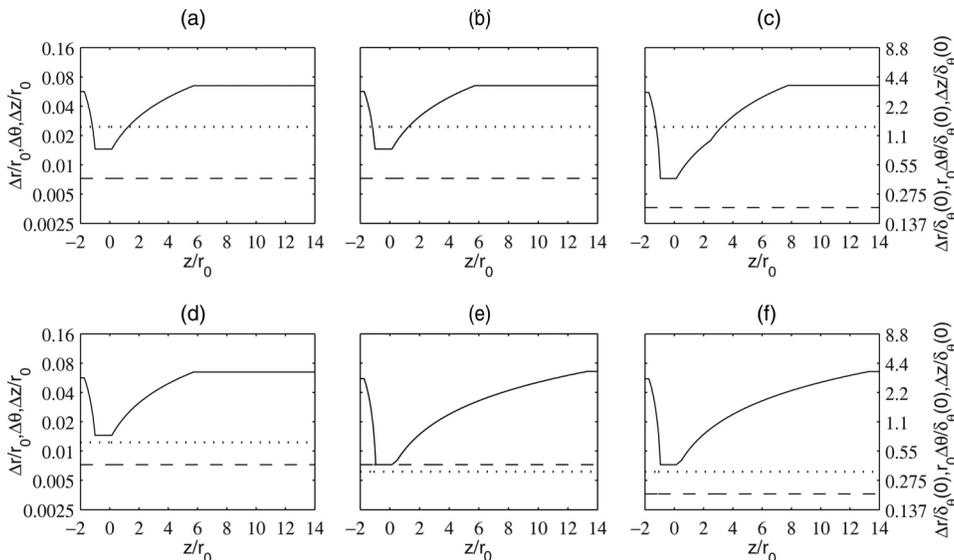
FIG. 3. Representation, in logarithmic scales, of the mesh spacings, —  $\Delta z$ , - - -  $\Delta r$ ,  $\dots\dots r_0\Delta\theta$ , at  $r=r_0$  in (a) Jetnoise256, (b) Jetring256, (c) Jetring256drdz, (d) Jetring512, (e) Jetring1024dz, and (f) Jetring1024drdz. The mesh spacings are normalized by  $r_0$  or  $\delta_\theta(0)$  as in Fig. 2.
