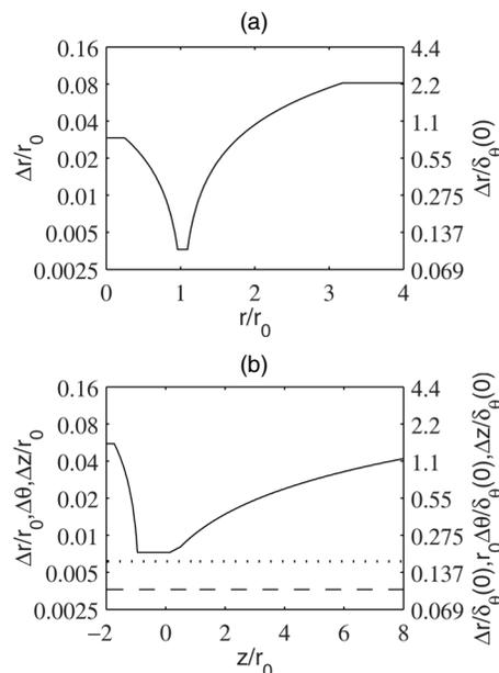
FIG. 4. Representation, in logarithmic scales, of the mesh spacings in Jetring1024drdz2 $\delta_\theta$ : (a)  $\Delta r$  as a function of  $r/r_0$ , (b) —  $\Delta z$ , - - -  $\Delta r$ , and  $\dots\dots r_0\Delta\theta$  at  $r=r_0$ . The mesh spacings are normalized by  $r_0$  or  $\delta_\theta(0)$  as in Figs. 2 and 3.
