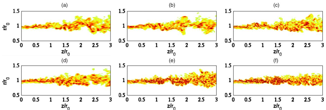
FIG. 6. (Color online) Snapshots in the  $(z, r)$  plane of vorticity norm just downstream of the pipe lip for (a) Jetnoise256, (b) Jetring256, (c) Jetring256drdz, (d) Jetring512, (e) Jetring1024dz, and (f) Jetring1024drdz. The color scale ranges up to the level of  $25u_j/r_0$ .
