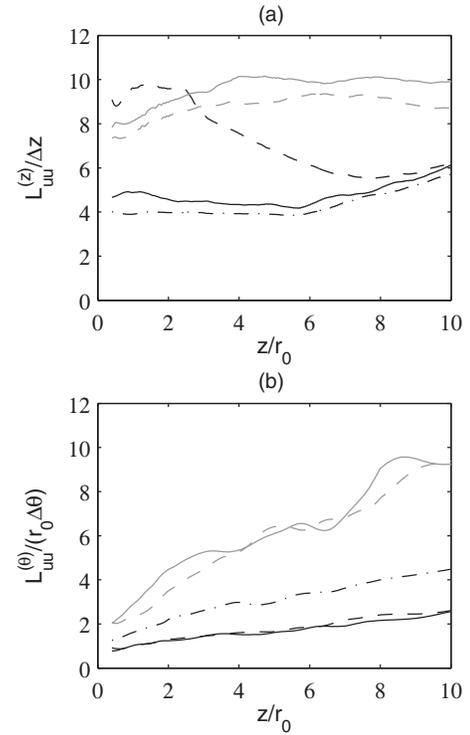
FIG. 27. Variations of the ratios (a)  $L_{uu}^{(z)}/\Delta z$  and (b)  $L_{uu}^{(\theta)}/(r_0\Delta\theta)$  between integral length scales calculated from  $u'_z$  and mesh spacings at  $r=r_0$  for — Jetring256, - - - Jetring256drdz, - · - · - Jetring512, gray solid line: Jetring1024dz, and gray dashed line: Jetring1024drdz.
