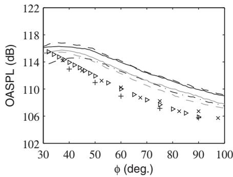
FIG. 24. Overall sound pressure levels at  $60r_0$  from the pipe exit as functions of the angle  $\phi$  relative to the jet direction for — Jetring256, --- Jetring256drdz, -·-·- Jetring512, gray solid line: Jetring1024dz, and gray dashed line: Jetring1024drdz. Measurements for jets at  $Re_D \geq 5 \times 10^5$ : + Mollo-Christensen *et al.* (Ref. 54),  $\times$  Lush (Ref. 55), and  $\triangleright$  Bogey *et al.* (Ref. 52).
