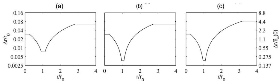
FIG. 2. Representation, in logarithmic scales, of the radial mesh spacing  $\Delta r$  normalized by the jet radius  $r_0$  or by the exit boundary-layer thickness  $\delta_\theta(0)$  in (a) Jetnoise256, Jetring256, Jetring512, and Jetring1024dz, (b) Jetring256drdz, and (c) Jetring1024drdz.
