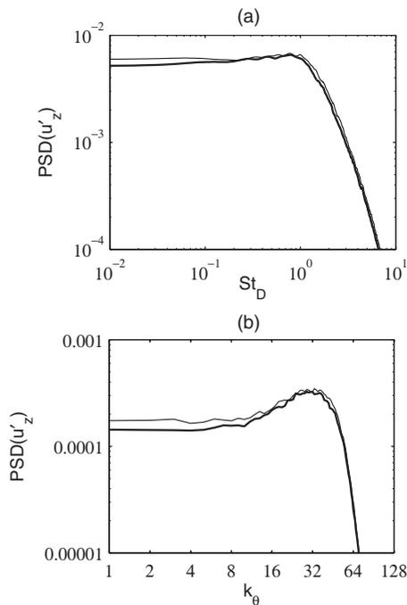
FIG. 11. Power spectral densities (PSDs) normalized by  $u_j$  of axial fluctuating velocity  $u'_z$  at  $r=r_0$  and  $z=0.4r_0$ , as functions (a) of the Strouhal number  $St_D=fD/u_j$  and (b) of azimuthal wave number  $k_\theta$  for — (thick line) Jetnoise256 and — (thin line) Jetring256.
