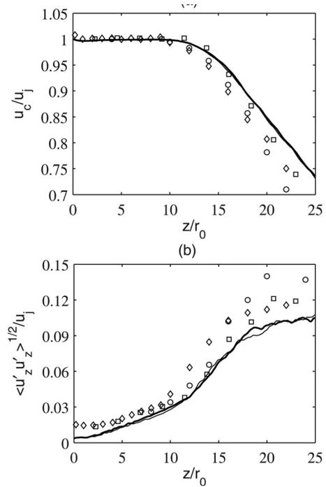
FIG. 13. Variations (a) of centerline mean axial velocity  $u_c$  and (b) of the rms value of fluctuating velocity  $u'_z$  at  $r=0$  for — (thick line) Jetnoise256 and — (thin line) Jetring256. Measurements for Mach 0.9 jets at  $Re_D \geq 5 \times 10^5$ :  $\circ$  Lau *et al.* (Ref. 50),  $\square$  Arakeri *et al.* (Ref. 17), and  $\diamond$  Fleury *et al.* (Ref. 49).
