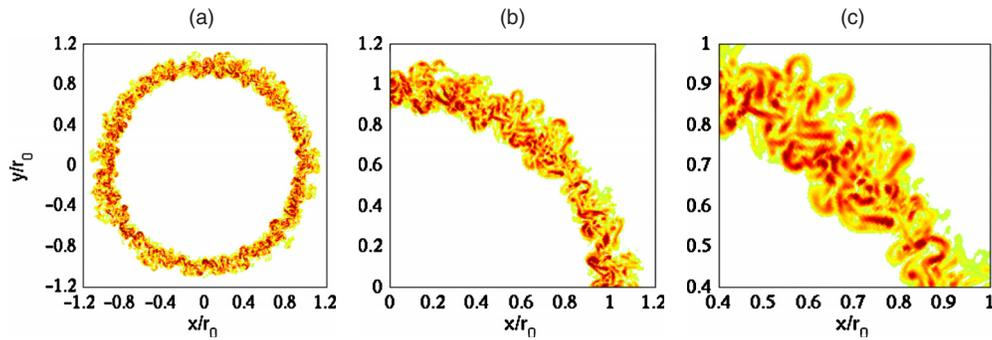
FIG. 7. (Color online) Snapshot in the  $(r, \theta)$  or  $(x, y)$  plane at  $z=r_0$  of vorticity norm for Jetring1024dz. Views over (a)  $-1.2r_0 \leq x, y \leq 1.2r_0$ , (b)  $0 \leq x, y \leq 1.2r_0$ , and (c)  $0.4r_0 \leq x, y \leq r_0$ . The color scale ranges up to the level of  $34u_j/r_0$ .
