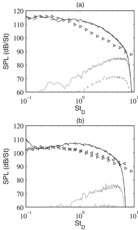
FIG. 26. SPLs at  $60r_0$  from the jet exit as functions of  $St_D = fd/u_j$  at the angles of (a)  $40^\circ$  and (b)  $90^\circ$  for Jetnoise256 with (black solid line) and without (gray solid line) jet flow and Jetring256 with (black dashed line) and without (gray dashed line) jet flow. Measurements for jets at  $Re_D \geq 7.8 \times 10^5$ :  $\triangleleft$  Tanna (Ref. 51) and  $\triangle$  Bogey *et al.* (Ref. 52).
