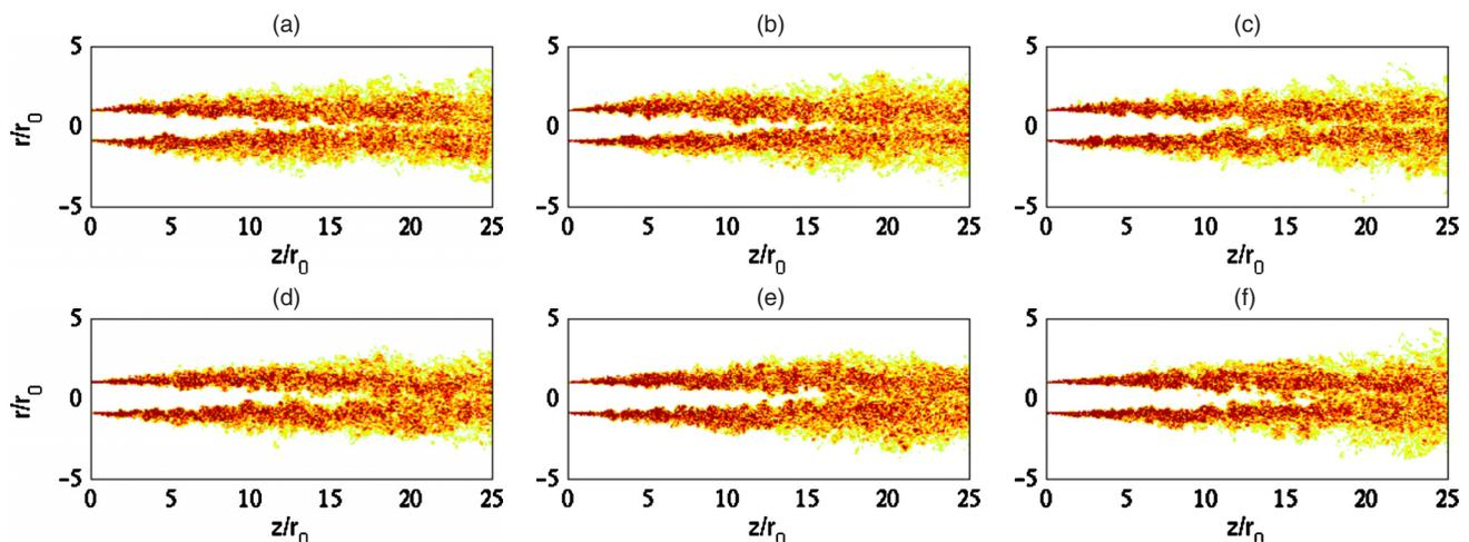
FIG. 8. (Color online) Snapshots in the  $(z, r)$  plane of vorticity norm up to  $z=25r_0$  for (a) Jetnoise256, (b) Jetring256, (c) Jetring256drdz, (d) Jetring512, (e) Jetring1024dz, and (f) Jetring1024drdz. The color scale ranges up to the level of  $5u_j/r_0$ .
