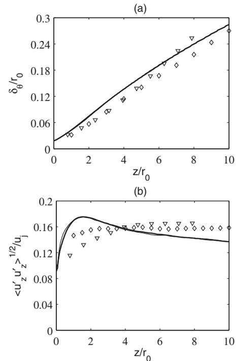
FIG. 12. Variations (a) of shear-layer momentum thickness  $\delta_\theta$  and (b) of the peak rms value of fluctuating velocity  $u'_z$  for — (thick line) Jetnoise256 and — (thin line) Jetring256. Measurements:  $\nabla$  Husain and Hussain (Ref. 13) for an initially turbulent shear layer and  $\diamond$  Fleury *et al.* (Ref. 49) for a Mach 0.9 jet at  $Re_D=7.7 \times 10^5$ .
