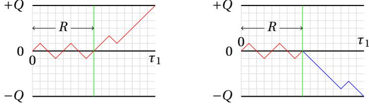
Figure 1: Illustration of the modified reflexion principle. The left figure depicts a detail of the up-crossing excursion, occurring between times 0 and  $\tau_1$ . The left figure depicts the details of a new admissible path bijectively obtained from  $Y$  by defining it as identical to  $Y$  for the times  $0 \leq t \leq R$  and then by reverting the flow of time and displacing the remaining portion of the path by  $-Q$ , as explained in the text.
