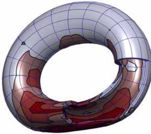
Figure 4: *case(b)*, the Von Mises criterion on the deformed torus meshed with one layer of regular hexahedric cells and a  $Q_2$  isoparametric FEM (with Getfem [26]).
