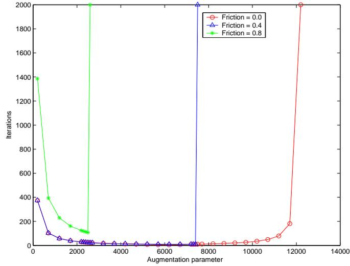
Figure 6: (*FPS*) influence of the augmentation parameter  $r$  for the torus with different values of the friction coefficient.
