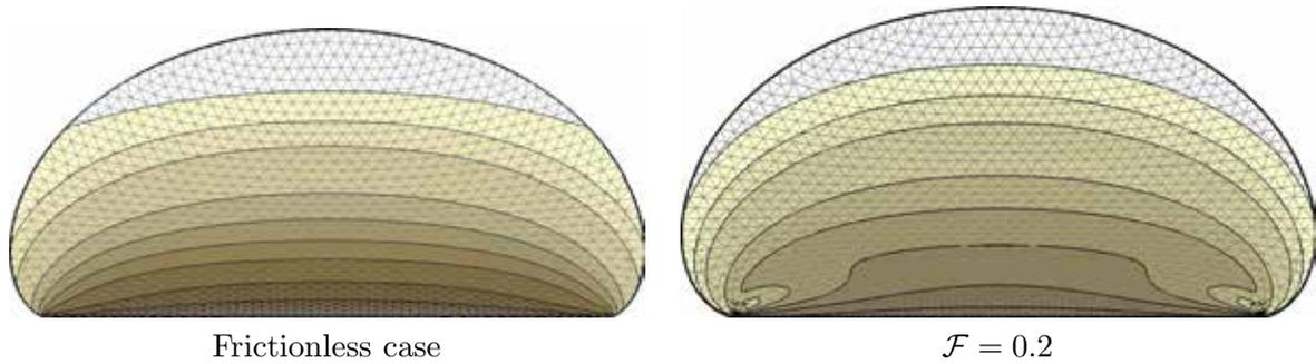
Figure 3: *case(a)*, the Von Mises criterion on the deformed disc meshed with  $P_2$  isoparametric FEM in frictional contact with a rigid foundation (with Getfem [26]).
