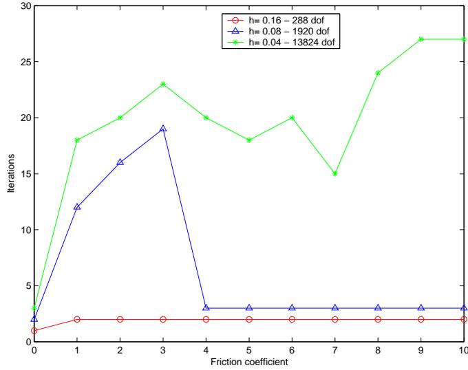
Figure 13: (*SSN*) influence of the friction coefficient for the torus with different mesh sizes.
