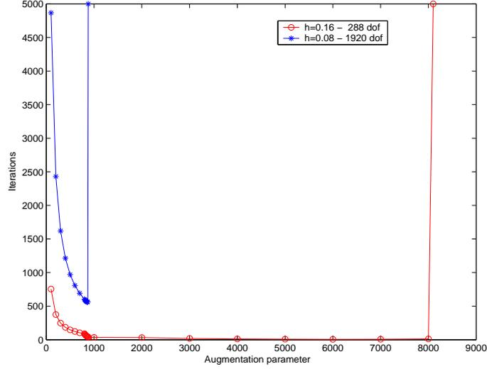
Figure 8: *(FPS) influence of the augmentation parameter  $r$  for the torus with different mesh sizes.*
