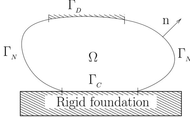
Figure 1: Elastic body  $\Omega$  in frictional contact.
