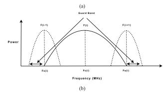
Fig. 4. An example showing channel bonding (a) when the channels are not bonded and (b) when three channels are bonded to create a single broadband bonded channel
