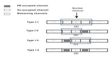
Fig. 2. Types of channels (Interior Free Channel Case): (a) Type I-1, higher bandwidth category, (b) Type I-2, higher bandwidth category, (c) Type I-3, higher bandwidth category, and (d) Type I-4, lower bandwidth category.
