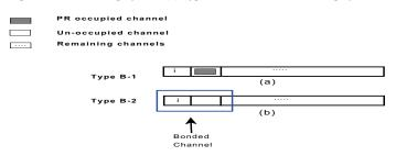
Fig. 3. Types of channels (Border Free Channel Case): (a) Type B-1, lower bandwidth category, and (b) Type B-2, higher bandwidth category.
