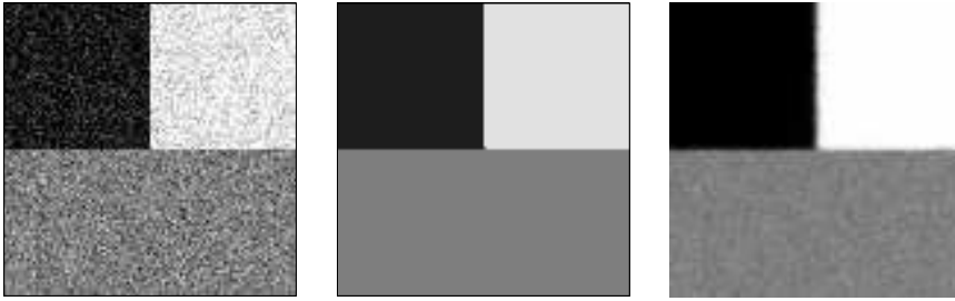
FIGURE 6. Greylevel image denoising with L^2 norm: original image (left, 100 \times 100 pixels), solution with 3 labels and \alpha = 10^{-3}\sqrt{n} (middle), solution taken from [28] (right).
