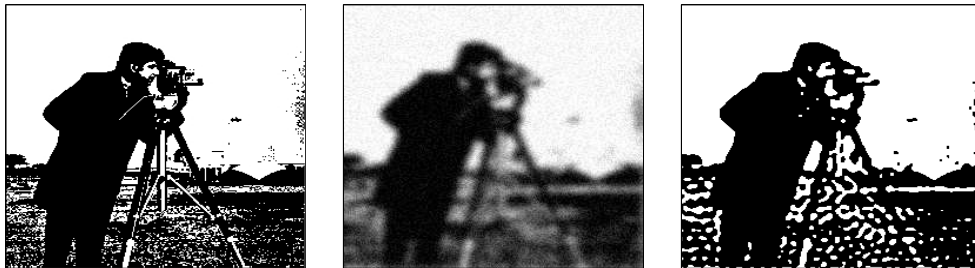
FIGURE 15. Deblurring and denoising: original image (left, 257 \times 257 pixels), damaged image with blur and noise effects (middle), reconstructed image for \alpha = 2.10^{-4}\sqrt{n} (right).
