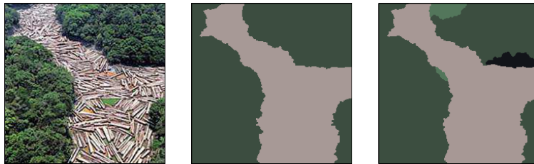
FIGURE 10. Unsupervised color image classification with L^1 norm, \alpha = 5 \cdot 10^{-3} \sqrt{n} : original image (left), obtained image with 2 labels (middle), obtained image with 5 labels (right)
