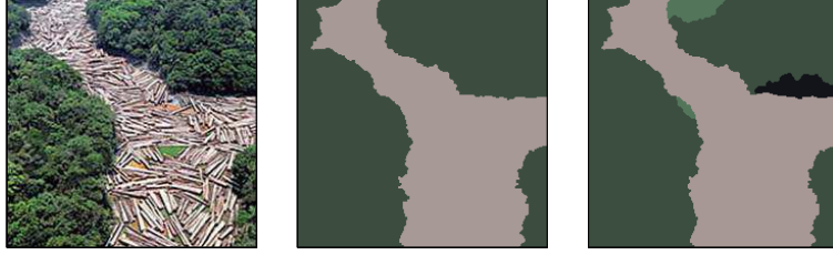
FIGURE 12. Unsupervised color image classification with L^1 norm, \alpha = 5.10^{-3}\sqrt{n} : original image (left, 231 \times 221 pixels), obtained image with 2 labels (middle), obtained image with 5 labels (right).
