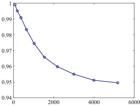
Figure 2. Mean-square convergence of the random effective stiffness matrix with respect to the number  $\nu$  of degrees of freedom of the finite element model for  $\delta = 0.4$ ,  $L_d = 0.1$  and for  $n_s = 900$ . Graph of function  $\nu \mapsto \text{conv}(n_s, \nu)$ . Horizontal axis  $\nu$ . Vertical axis  $\text{conv}(n_s, \nu)$ .
