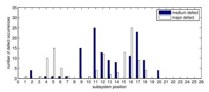
Fig. 5 Number of medium (blue) and major (white) defect occurrences with respect to the capacitor positions for track circuits containing 25 capacitors and according to the REF labeling.
