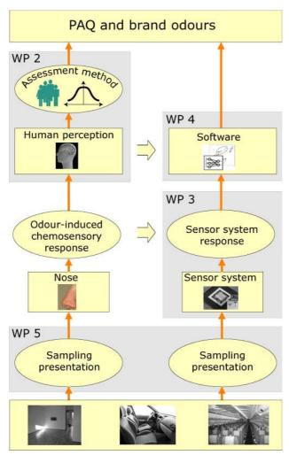
Figure 1: Parallelism of the human perception of air quality and brand specific odours on the left hand side and the sensor system development on the right hand side
