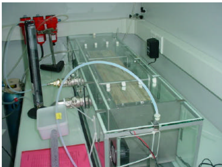
Figure 1 : 51 litre glass chamber used for the test
