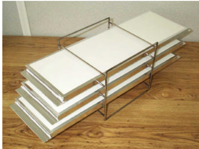
Figure 2: test specimens prepared from particleboard with melamine on top
