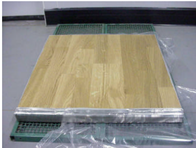
Figure 6 : multi-layer parquet floor glued on a concrete substrate
