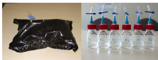
Figure 1 A modified Tedlar ® bag and the modified butanol reference bottles.
