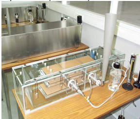
Figure 1. Emission test chamber used by CSTB (Climpaq, 50 L)
