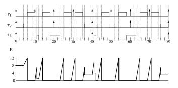
Figure 10. UPPAAL Feasible Schedule With Minimal Change Mode of the Battery: Battery  $\mathcal{B}(12,7)$  and  $e_1 = 3, e_2 = e_3 = 1$
