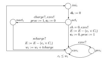
Figure 5. Adding Energy Consumption to the Timed Automaton Task<sub>i</sub>
