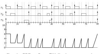
Figure 1.  $EDF_{asap}$ : Battery  $\mathcal{B}(10,2)$  and  $e_1 = e_2 = e_3 = 1$
