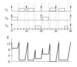
Figure 7.  $PFP_{2,1,3}$  Schedule: Battery  $\mathcal{B}(13,7)$  and  $e_1 = 3, e_2 = e_3 = 1$
