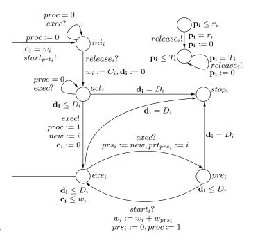
Figure 2. Timed Automaton Model for a Task  $\tau_i$
