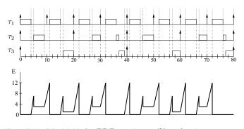
Figure 8.Not Schedulable for  $EDF_{asap}$ : Battery  $\mathcal{B}(12,7)$  and  $e_1 = 3, e_2 = e_3 = 1$
