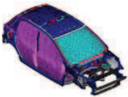
Figure 28. Mean finite element model of the internal acoustic cavity with incompatible mesh on the acoustic-structure coupling interface.
