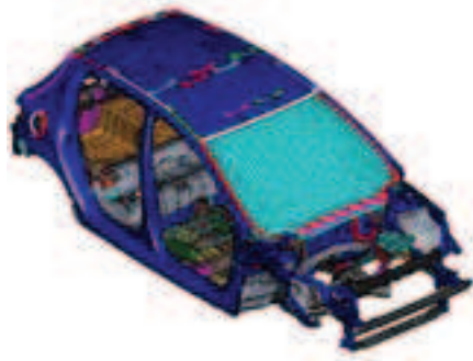
Figure 27. Mean finite element of the structure (car body).
