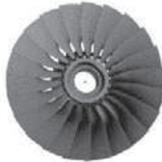
Figure 12. Finite element mesh for the 22 blades fan stage
