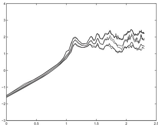
Figure 14. Nonlinear case:  $\log_{10}$  of the random normalized response spectrum (vertical axis) as a function of  $\log_{10}$  of the frequency for the  $[1, 200]Hz$  frequency band. Deterministic response of the mean model (mid irregular thin solid line). Mean value of the model with random uncertainties (mid smoothed thin solid line). Lower and upper envelopes of the confidence region (lower and upper thick solid lines). Extreme value statistics (lower and upper thin solid lines).
