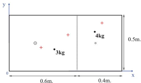
Figure 8. Nonhomogeneous structure: rectangular plate in bending mode with 2 point masses ( $\bullet$ ) and 3 springs ( $+$ ). Excitation: point force ( $\odot$ ). Response: normal displacement ( $\circ$ ).
