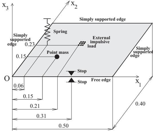
Figure 11. Geometry of the structure
