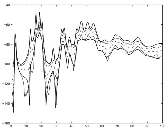
Figure 10. Modulus in dB of the stochastic cross-frequency response function in frequency band  $[1, 100] \text{ Hz}$  (horizontal axis). Mean response (thin dashed line), confidence region corresponding to a probability level of 0.95 (thick solid lines), extreme value statistics (thin solid lines).
