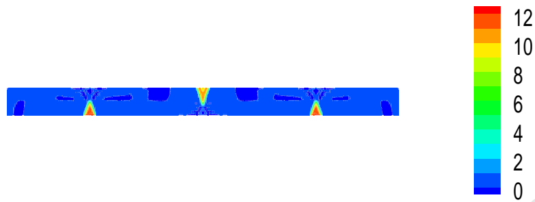
Figure 10: Light bar: divergence of the velocity vector after the collision for U^- = 6.25 \text{ m/s} . The opening fractures are represented by zone with high values of \text{div}(\vec{U}^+) .
