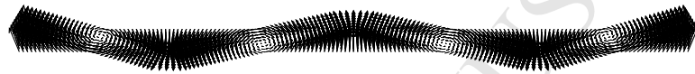
Figure 11: Light bar: velocity \vec{U}^+ after the collision for U^- = 12.5 \text{ m/s} . The bar is broken into four pieces.
