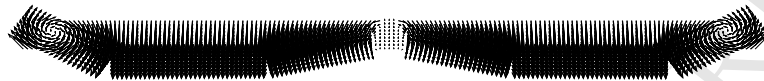
Figure 6: Heavy bar: velocity \vec{U}^+ after the collision for U^- = 3.125 \text{ m/s} . The bar is broken into seven pieces.
