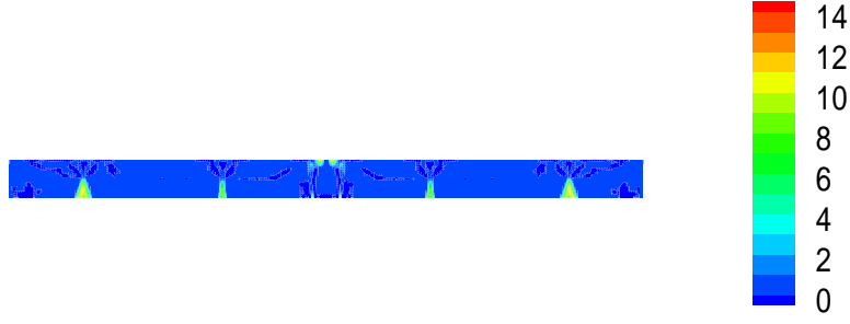
Figure 7: Heavy bar: divergence of the velocity vector after the collision for U^- = 3.125 . The opening fractures are represented by zone with high values of \text{div}\vec{U}^+ .
