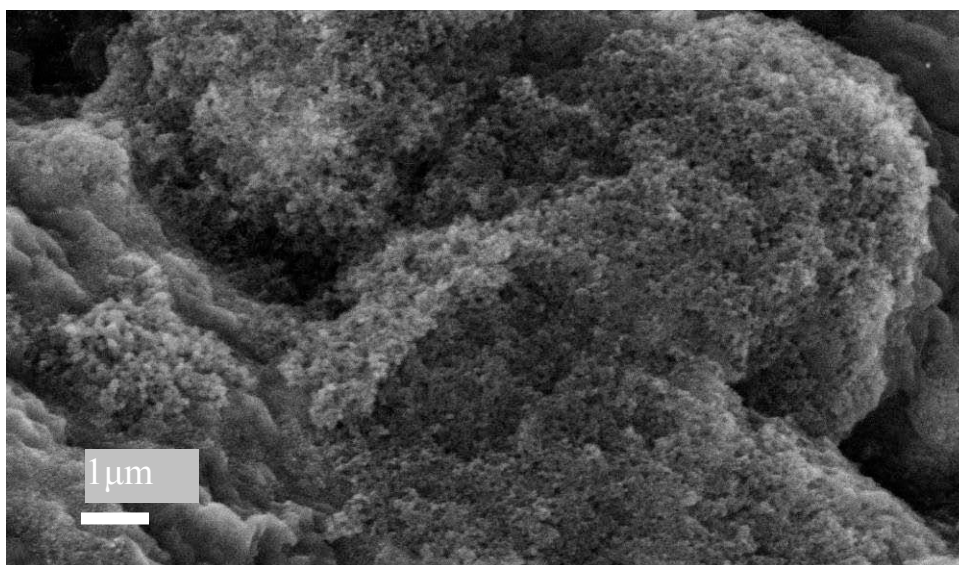
Figure 5. SEM image of SWNTs after Procedure 2 (described in the text) showing the nanotubes have primarily been converted to amorphous carbon. (FINAL PRODUCT 2)
