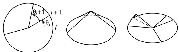
Figure 8. Illustration of local flat foldability theorem, for the flat unfolded state (left), and two non-flat states (center and right).
