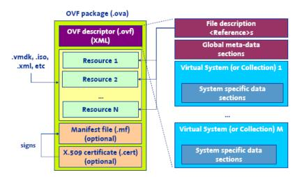
Figure 4.1: OVF package and descriptor structure
