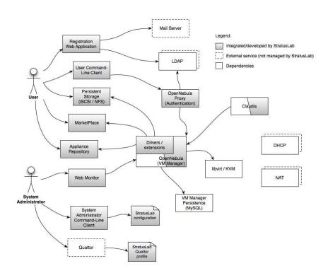
Figure 3.1: StratusLab Services and Components
