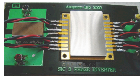
Figure 14: A JFET-based, 540 V, 15 A, 3-phase inverter in a single package with an external DC capacitor.
