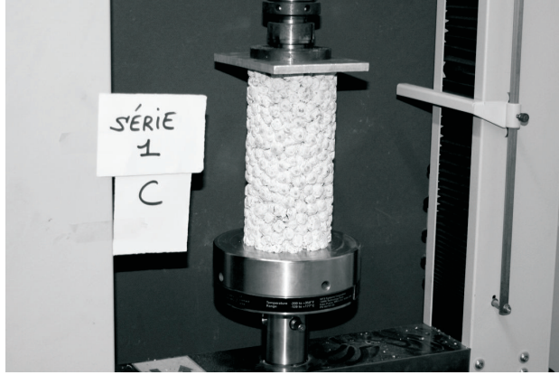
Figure 2: An experimental sample of cylindrical shape subjected to simple compression test.
