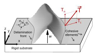
FIG. 2 (color online). Model for thin film buckling and delamination: a nonlinear plate on a rigid substrate with a mixedmode cohesive zone model for the adhesive interface.
