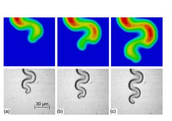
FIG. 1 (color online). Telephone cord propagation: comparison between numerical results (top) and optical measurements (bottom). Configurational instability induces a sag at the front, resulting in the pinning of the outer edge of the buckle in almost pure shear. The blister grows further around this pinning point thus changing the direction of rotation.
