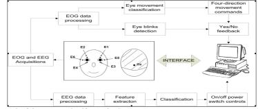
Figure 1. Framework of the proposed self-paced BCI system.
