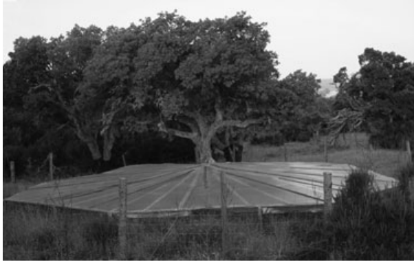
Fig. 1. Cork oak tree with its root zone covered by a plastic roof for rainfall interception.
