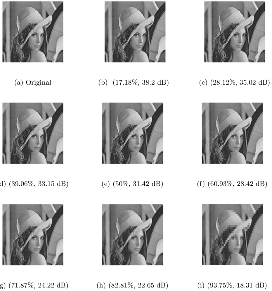
Fig. 10: Simulation of image compression using the VHDL model
