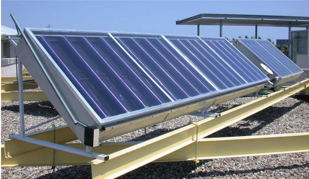
**Figure 5:** Prototype built at the PROMES laboratory in Perpignan (South of France). The solar collector of pole  $b_2$  is shown on the left side and is separated by the pyranometer from the solar collector of pole  $a_2$  on the right side.
