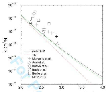
Figure 1. Thermal rate constant k(T) of the  $H + CH_4 \rightarrow H_2 + CH_3$  reaction [18, 19]: accurate quantum mechanical results and transition state theory results calculated on an accurate ab initio PES are displayed together with experimental results. Results obtained for a the PES which is based only on ab initio data from geometries located at the minimum energy path (MEP) are also shown.
