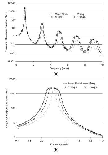
Figure 2. (a) Frobenius norm of the frequency response function matrix, (b) same, zoomed. Mean model 1.Constrained Model ("2Freq"), unconstrained models with higher ("1FreqHi") and lower ("1FreqLo") level of variations.
