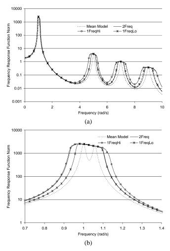
Figure 4. (a) Frobenius norm of the frequency response function matrix, (b) same, zoomed. Mean model 2.Constrained Model ("2Freq"), unconstrained models with higher ("1FreqHi") and lower ("1FreqLo") level of variations.
