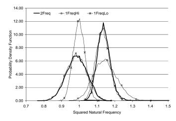
Figure 3. Probability density functions of the squared first and second natural frequencies. Mean model 2. Constrained Model ("2Freq"), unconstrained models with higher ("1FreqHi") and lower ("1FreqLo") level of variations.
