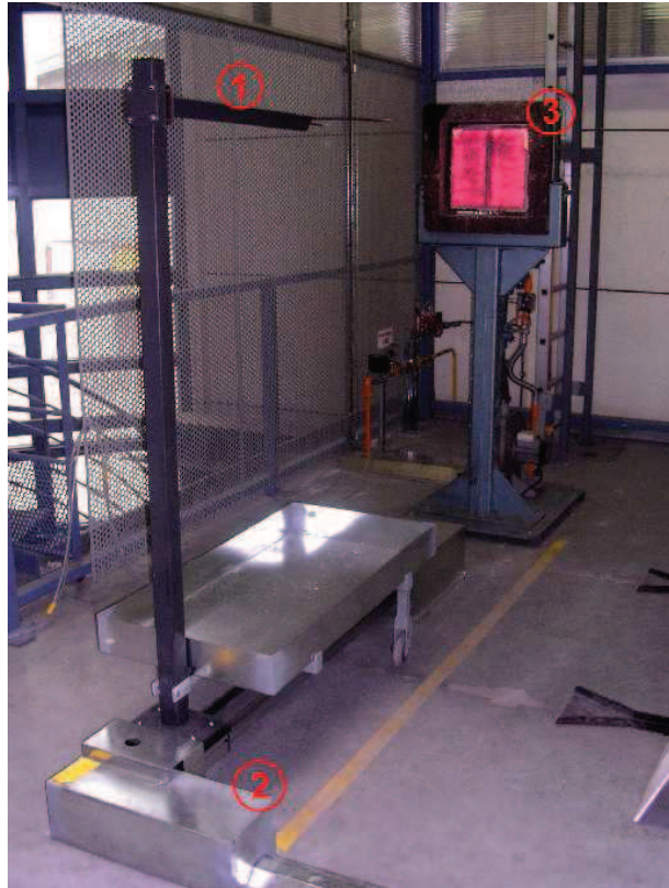
Figure 1: Thermal load bench composed of: ①: Specimen holder, ②: mobile cart and ③: radiant panel.
