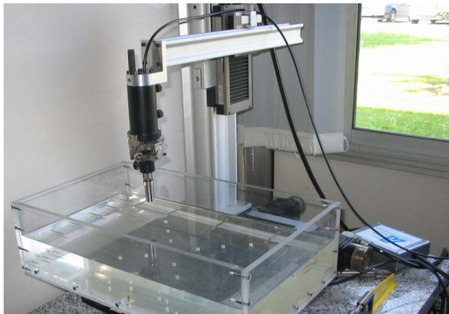
Figure 6. Experimental device: robotic displacement and ultrasonic sensor.
