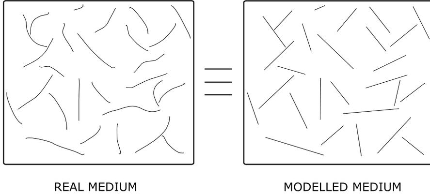
Figure A.1. Schematic of the equivalence between real medium (curved fibers) and modelling (straight fibers).
