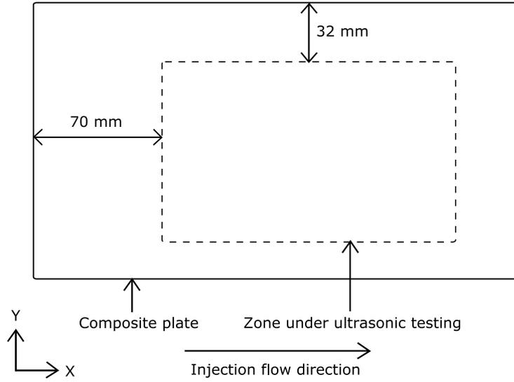
Figure 7. Composite plate and zone under experimental investigation.
