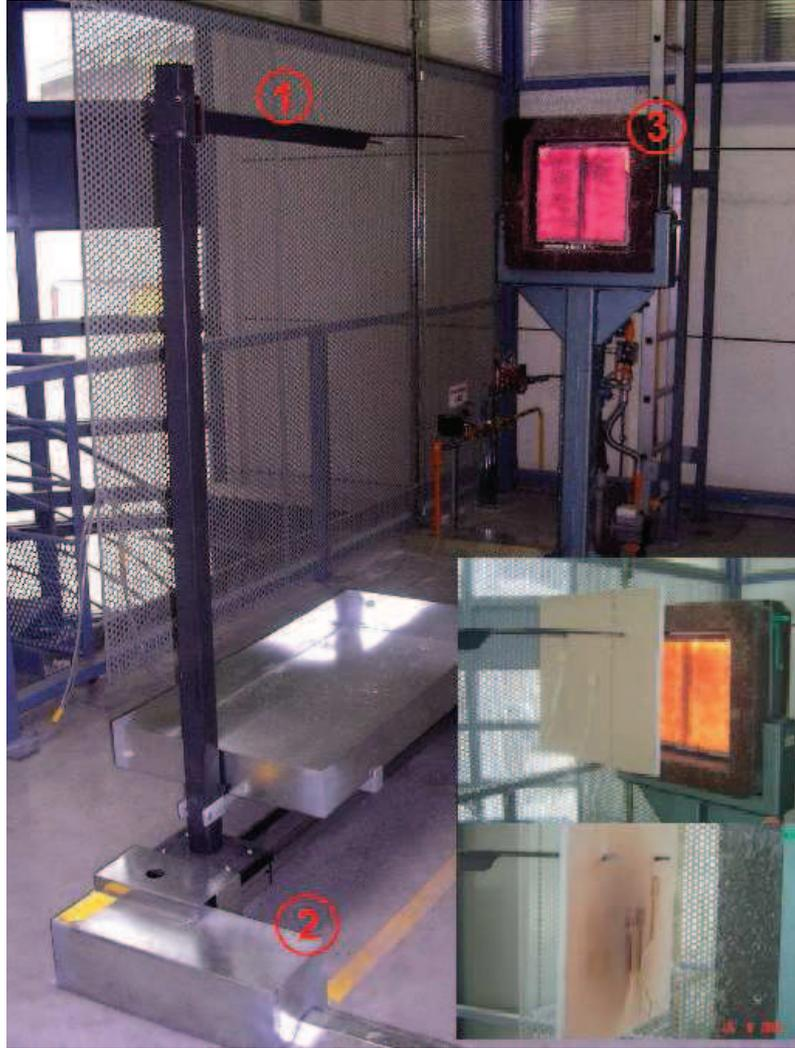
Figure 2: Thermal load bench composed of: ①: Specimen holder, ②: mobile cart and ③: radiant panel.
