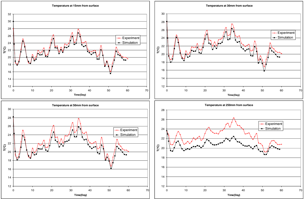
Figure 7: Evolution of temperature at different depth from the wall surface (south borehole).
