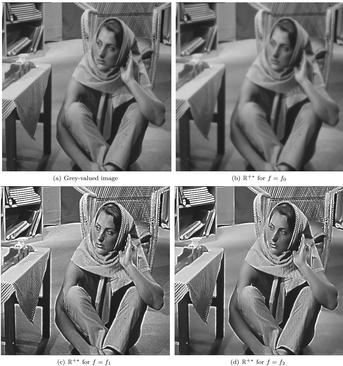
Fig. 1 Grey-valued image diffusions from heat equations of generalized Laplacians parametrized by a function f and the unique dual representation of \mathbb{R}^{+*} on \mathbb{R} .
