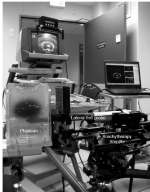
FIG. 11. Prostate phantom with a horizontal cylindrical rectum, being used with a side-fire US probe during a mock brachytherapy test.
