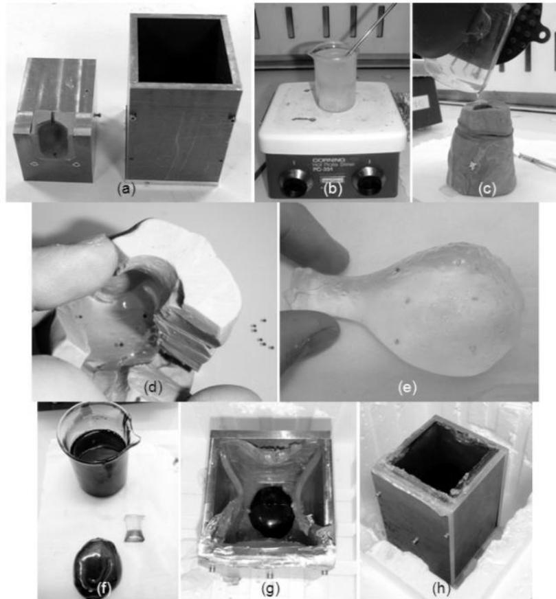
FIG. 2. Steps during construction of the prostate phantom. (a) Mould used to shape the outer frame of the phantom. (b) Heating of the PVC mixture. (c) Pouring the molten PVC into the prostate mould. (d) Placing the targets onto the first layer of the prostate. (e) The final prostate shape. (f) Coating the prostate with an echogenic stained PVC mixture. (g) Putting the prostate in place inside the frame. (h) Allowing the phantom to cool overnight.
