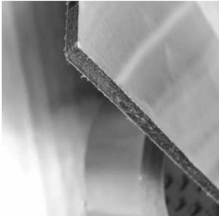
Figure 1: Dupont de Nemours PCM composite wallboard.
