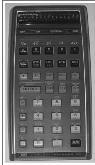
Figure 15. Electronic pocket calculator HP-65.
