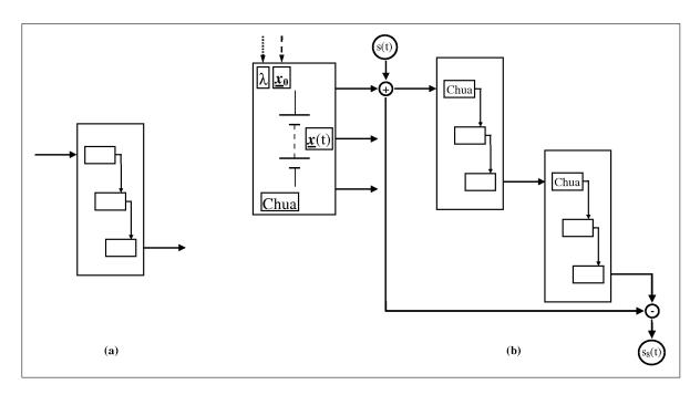
Fig. 16. (a) Cascader symbol. (b) Two cascading receivers combined.
