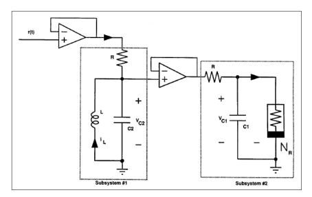
Fig. 3. Practical realization of the receiver. The first subsystem is a partial Chua's circuit consisting of the  $(v_{C_2}, i_L)$ -subsystem driven by the transmitted signal r(t). The second subsystem is a partial Chua's circuit consisting of the  $(v_{C_1})$ -subsystem driven by the transmitted signal  $v_{C_2}^{(1)}$ . The triangular symbols are OpAmps which decoupled the systems, acting as the signal drive elements, from.<sup>15</sup>
