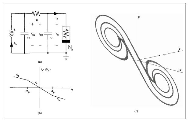
Fig. 1. (a) Realization of Chua's circuit from.<sup>5</sup> (b) Three-segment piecewise-linear v-i characteristic of nonlinear resistor in Chua's circuit. (c) Chua attractor.
