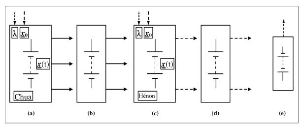
Fig. 7. Generators. (a) Continuous generator (Chua's circuit, expanded symbol). (b) Simplified continuous generator. (c) Discrete generator (Hénon map, expanded symbol). (d) Simplified discrete generator. (e) 1-dimensional logistic generator.
