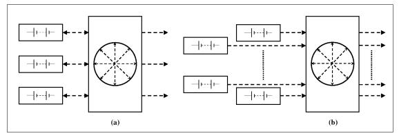
Fig. 11. (a) Circuit of ultraweak coupling of three 1-dimensional chaotic maps. (b) Circuit of ultraweak coupling of p 1-dimensional chaotic maps.
