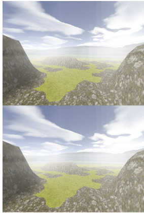
Figure 7: Quality difference when removing a layer of details. Above : Haar fog with a resolution of 32 \times 32 . Below : Same fog, minus the lower layer of details.
