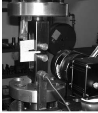
Fig. 9. Compact tension test specimen and DIC system.
