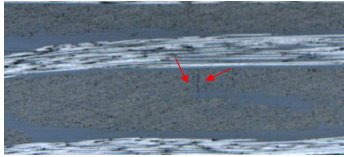
Damage location at 2-1(nested yarn)
