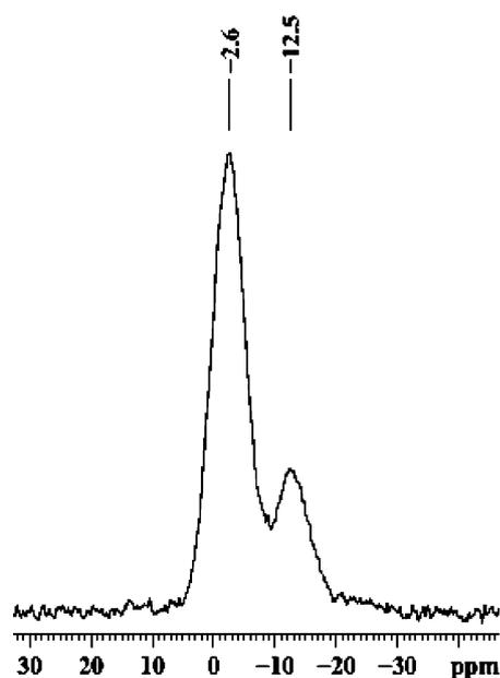
**Fig. 7**  $^1\text{H}$ - $^{31}\text{P}$  CP MAS NMR of PCP. The peak at –2.6 ppm corresponds to the phosphonic acid group of (III) and the peak at –12.5 ppm corresponds to the dimer of the grafted moiety (Fig. 1)
