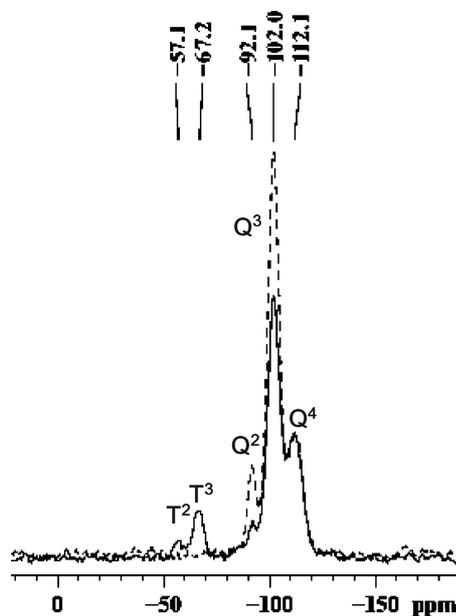
**Fig. 5**  $^1\text{H}$ - $^{29}\text{Si}$  CP MAS NMR of PCP (continuous line) and native silica (dashed line). The appearance of peaks  $\text{T}^2$  and  $\text{T}^3$  and the decrease of peaks  $\text{Q}^2$  and  $\text{Q}^3$  confirmed the polymeric bonding reaction of (II) (Fig. 1)
