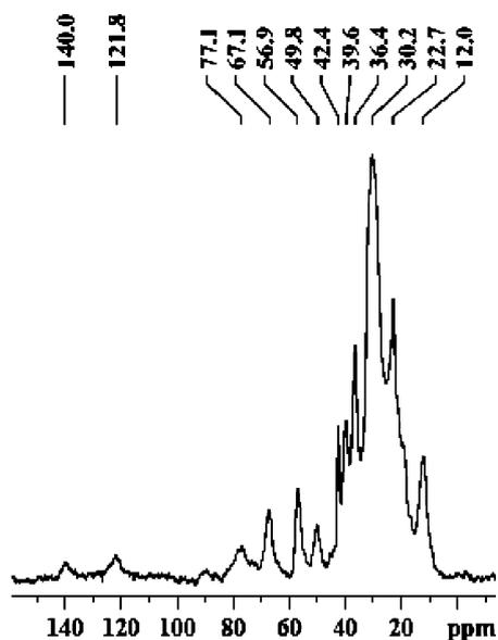
**Fig. 6**  $^1\text{H}$ - $^{13}\text{C}$  CP MAS NMR of PCP. Peaks at 140.0 and 121.8 ppm correspond to the olefin, peaks at 77.1 and 67.1 ppm correspond to the carbons directly bonded to the phosphonic acid group, peaks in the 56.9–12 ppm range correspond to the cholesteryl and alkyl moieties, and the peak at 12 ppm corresponds to the carbon directly bonded to the silicone (Fig. 1)
