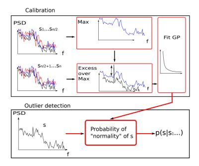
Figure 1: Peak-over-threshold detection algorithm.
