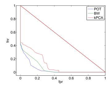
Figure 7: ROC curves for Algorithms POT, BW and kPCA. Faulty test data recorded after n = 2 days of operation. The diagonal can be interpreted as the output of a detector which would randomly trigger an alarm, ignoring all the data.
