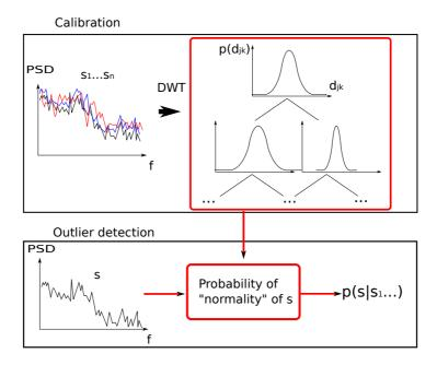
Figure 2: Bayesian detection in a wavelet basis (BW).
